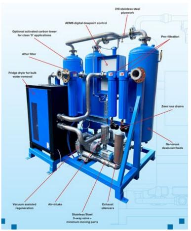
Hi-Plex dual technology dryers combine Hi-line's established refrigeration and PSA (Pressure Swing Adsorption) air treatment technologies, creating an energy-efficient system at low capital cost compared with standard heat-regeneration desiccant air dryers.
